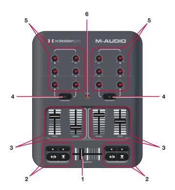
While X-Session Pro may look like a traditional DJ mixer, keep in mind that all of the buttons, knobs, and faders are actually sending out MIDI data. This means that you can use X-Session Pro to control more than just DJ applications. For example, the buttons, sliders, and knobs can be used to control a virtual instrument or a DAW sequencer. Refer to your software's user guide to learn how to map X-Session Pro's controls to various functions within the application.
